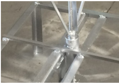
Figure 6. Mounted roller at the bottom of solar tracker system
