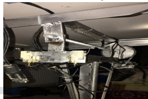
Figure 5. Mounted limit switches at the solar tracker system
